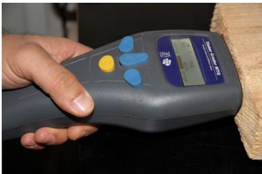
MTG is applied to timber with rectangular cross-sections shaped by sawing, planing or other methods and with cross-sectional dimensions complying with EN 336. Usually the dimension's guidelines are: width 36 – 110 mm; height 63 – 242 mm and length 1500 – 8000 mm.
